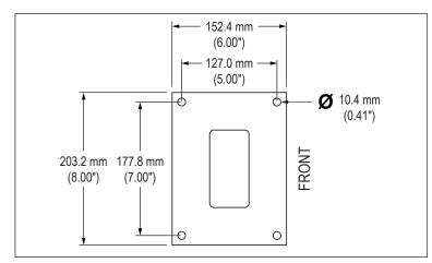
FIGURE 1 - PEDESTAL BASE PLATE
